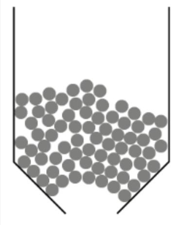
An illustrated cross-section example of feedstock bridging.
