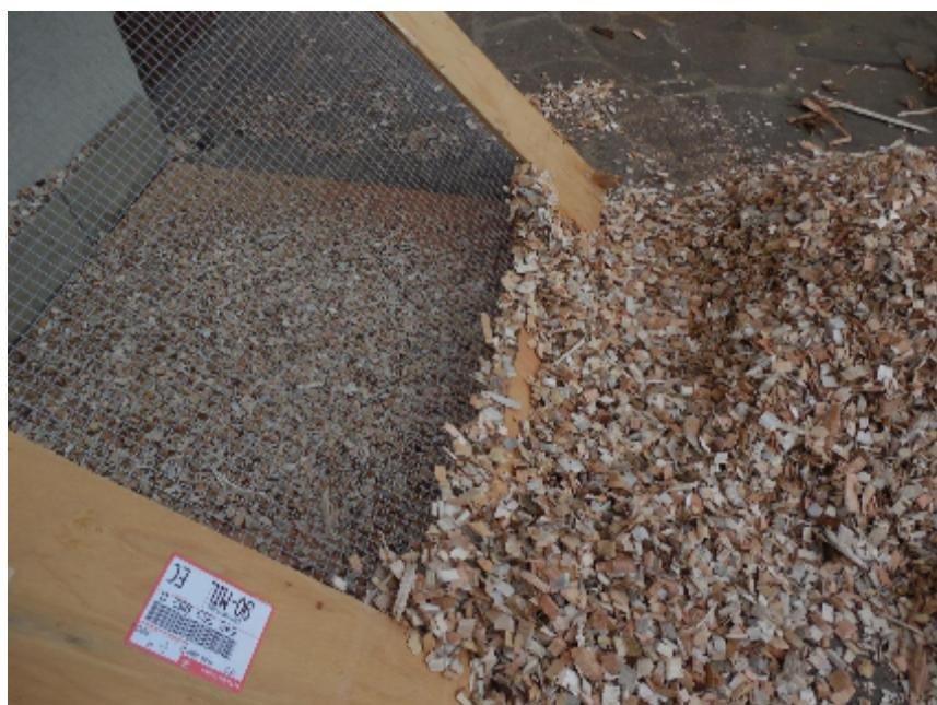
*Sifting with the  $\frac{1}{2}$ " screen to remove undersized pieces and fines. These fall through the screen.*
