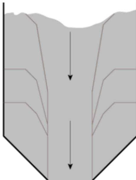
Mass flow is preferable to funnel flow; feedstocks that strongly exhibit funnel flow are prone to rat-holing and bridging. **Both of these forms of fuel jams leave feedstock deceptively visible through the viewport on the hopper**; if the low fuel alarm is sounding, but the hopper viewport shows feedstock, there is probably a fuel jam of some sort in the hopper.
