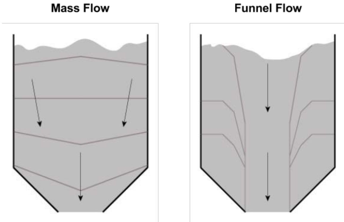
Mass flow is preferable to funnel flow; feedstocks that strongly exhibit funnel flow are prone to rat-holing and bridging. ***Both rat-holing and bridging fuel jams leave feedstock deceptively visible through the viewport on the hopper;*** if the low fuel alarm is sounding, but the hopper viewport shows feedstock, there is probably a fuel jam of some sort in the hopper.
