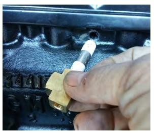
1C. If the nipple stays in the block, remove it using the included screw extractor. Tap it lightly into the pipe nipple and use the 8mm wrench to turn CCW.
