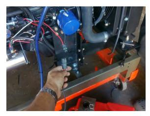
3A. Disconnect the syngas-supply corrugated gas line from the top of the governor, and securely attach the Fuel Injection unit onto the top of the governor in place of the gas line.
