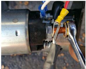
2C. Remove the 8mm nut on the small stud on the back of the starter, and install the white wire with small ring terminal on top of the one already there, and replace the nut.
