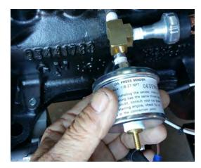
1E. If needed apply PTFE to threads and install the new Oil Pressure Safety Switch (APL Part # 185-00016 A) into the side outlet.
