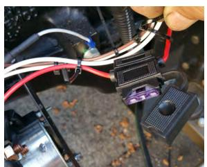
2E. Plug the timing adjust plug with the blue gasket into the open socket on the distributor. This connection will automatically readjust the timing for gasoline.
