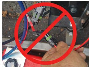
4C. Clip the leads, red to the large stud on back of starter, black to bare metal on the engine, pump will start. Watch the fuel fill the hose, and remove clips as soon as all air is purged.
