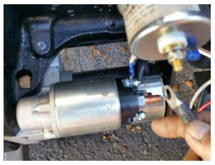
2A. Attach the black 3-wire plug to the oil pressure sender. Note: plug will not be able to bottom out on the switch and some slight bending of the terminals will occur.
