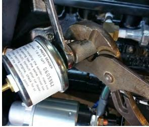
1A. Remove the 8mm nut and brown wire from the existing oil sender, and remove the sender using the 14mm open end wrench.
