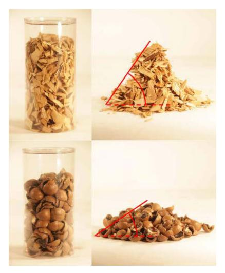
A comparison of the angle of repose of wood chips and of macadamia nut shells. The greater angle of repose of the wood chips correlates a greater risk of bridging and rat-holing.
