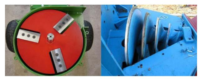
An example of the chipping mechanisms of a disc chipper compared to a screw auger chipper.
