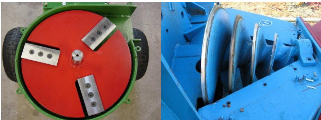
*An example of the chipping mechanisms of a disc chipper compared to a screw auger chipper.*
