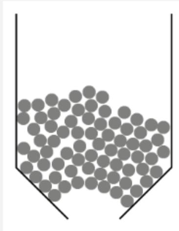
*An illustrated cross-section example of feedstock bridging.*
