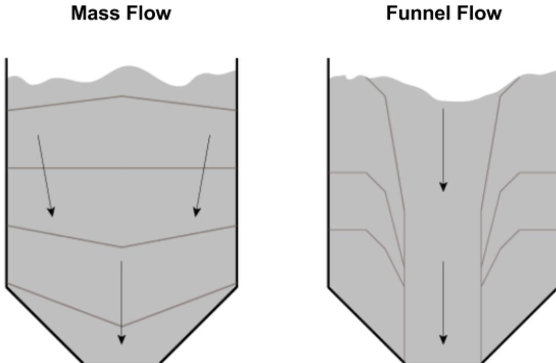
Mass flow is preferable to funnel flow; feedstocks that strongly exhibit funnel flow are prone to rat-holing and bridging. ***Both of these forms of fuel jams leave feedstock deceptively visible through the viewport on the hopper;*** if the low fuel alarm is sounding, but the hopper viewport shows feedstock, there is probably a fuel jam of some sort in the hopper.
