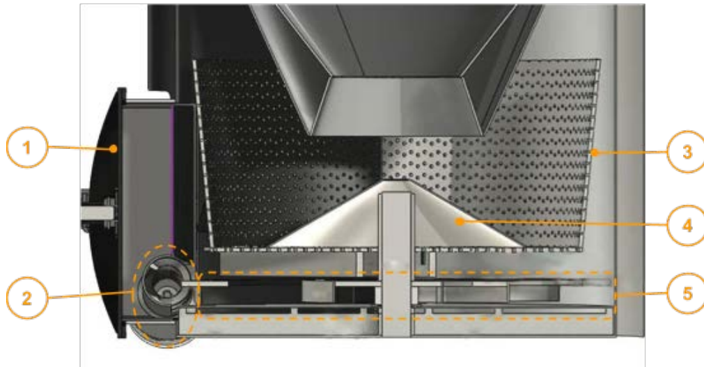
Transparent top view of ash handling system
