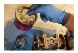
7. Using any standard automotive grease, use your finger to lubricate the throttle shaft with a small fingertip full of grease.
