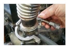
2. Loosen the two sani clamps and remove the whole governor.
