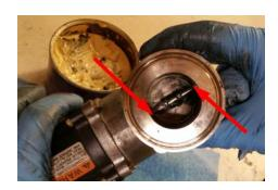
8. Push the grease into where the shaft goes into the housing, and make sure to do it to both the right and left sides both top and bottom.
