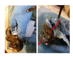
5. Wipe off plate & throat, then push a half sheet of paper towel or small rag all the way through both sides a few times to remove the softened soot & tar.
