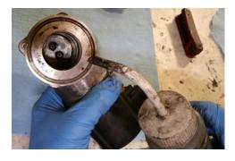
3. Use squirt bottle and solvent used for lighting gasifier to rinse both sides of the throttle.
