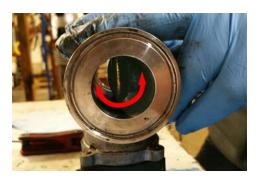
4. Work the throttle plate open and closed while wet with solvent until it moves smoothly and doesn't stick, move roughly or feel "crunchy."
