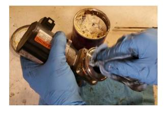
9. Use a paper towel or rag to wipe off excess grease. Get as much as possible, only the grease pushed into the shaft is useful.
