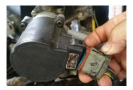
1. Disconnect plug from governor by pushing down the two locking tabs and pulling it away.
